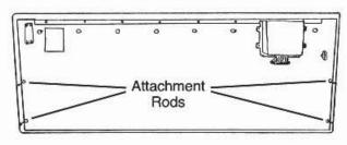
Pictured are the attachment rods on the piano bottom.
